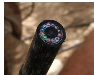
Photo: A section of 144-strand fiber-optic cable. Each strand is made of optically pure glass and is thinner than a human hair. Picture by Tech. Sgt. Brian Davidson, courtesy of US Air Force.
